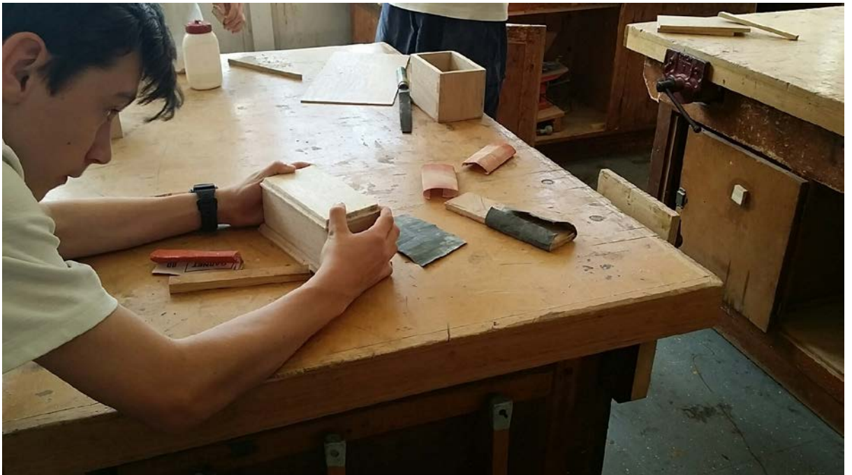
Year 9 Timber students have been designing their own jewellery boxes using advanced joinery such as finger joints to create their custom designs.
